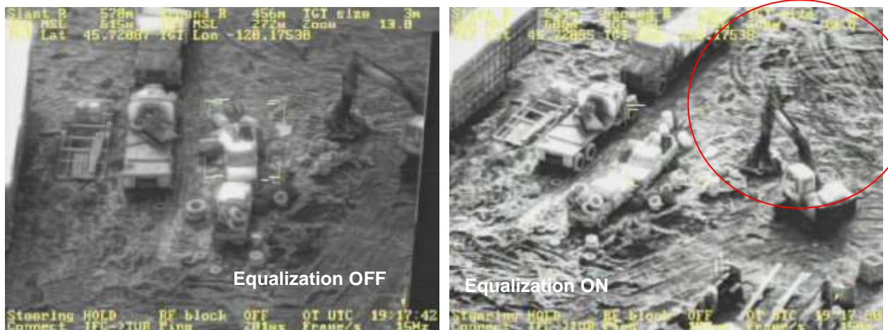
Equalization reveals vehicle tracks in top right corner of the image
